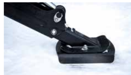
There are additional plates available for the KESLA 300 series A and Flapdown stabilizer legs.
